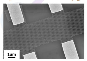
2. Magnetic plasmonic structure fabricated by i LiNE
